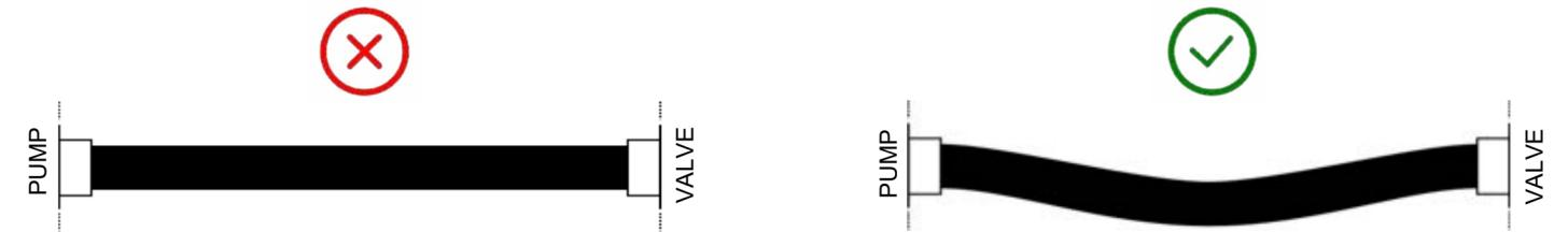
N.B. Assemble the hose so as to withstand length variations due to working pressure, pump movements and related tolerances. Avoid live assemblies.
